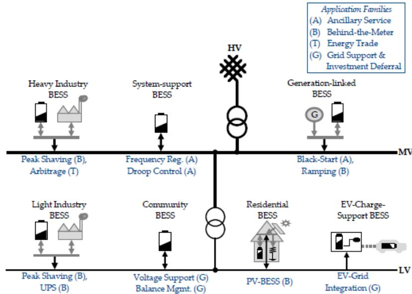
**Figure 7.** Variant types of stationary battery storage systems (black color) grouped according to their integration to Low-Voltage (LV) and Medium-Voltage (MV) grid levels. Typical applications are listed in blue color, letters in brackets link to *application families* as defined in the figure legend. Overlying High-Voltage (HV) connection and transformer links are depicted schematically.
