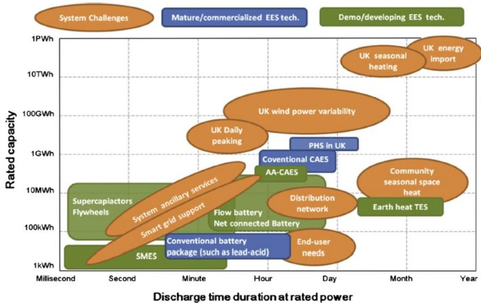
Fig. 1. Electrical energy storage technologies with challenges to the UK energy systems [4,6,7-9].
